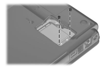
Where used: 2 screws that secure the WLAN module to the system board
